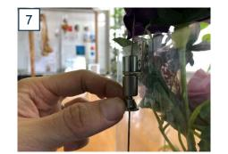
To move downward, pull down the part attached to the side of the exhibit with the grip attached. It locks at the released position.
