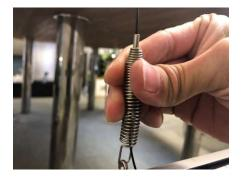
Insert the spring + attachment side of the wire from the end (hole) of the bottom rail, and do not push the tip pin, but pull the wire until it has an appropriate tension while lifting only the spring part. The wire is locked at the point where it is pulled, and the excess wire can be cut or placed inside the rail. The length of the wire can be adjusted by pushing the pin at the tip of the spring part while lifting the spring part upward. Since the wire has a lot of tension, repeat it many times
